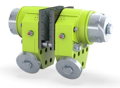
An extension of the brake piston through the adjustment nut gives an easy visual way to tell when adjustment is needed. The SKP 140 is equipped with "Easy Adjustment-arrangement" as standard.
